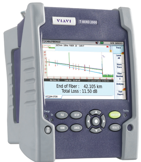
VIAVI T-BERD/MTS-2000 can integrate a VFL to detect bends or breaks
