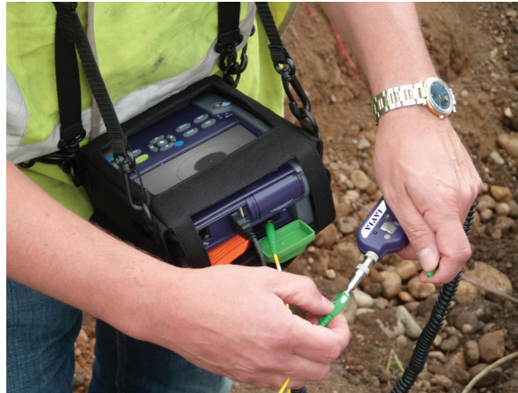
VIAVI T-BERD®/MTS-2000 with OTDR and digital microscope
